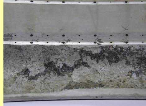
Notice the damage on the injector head. There is some room for doubt about HFI, though small
