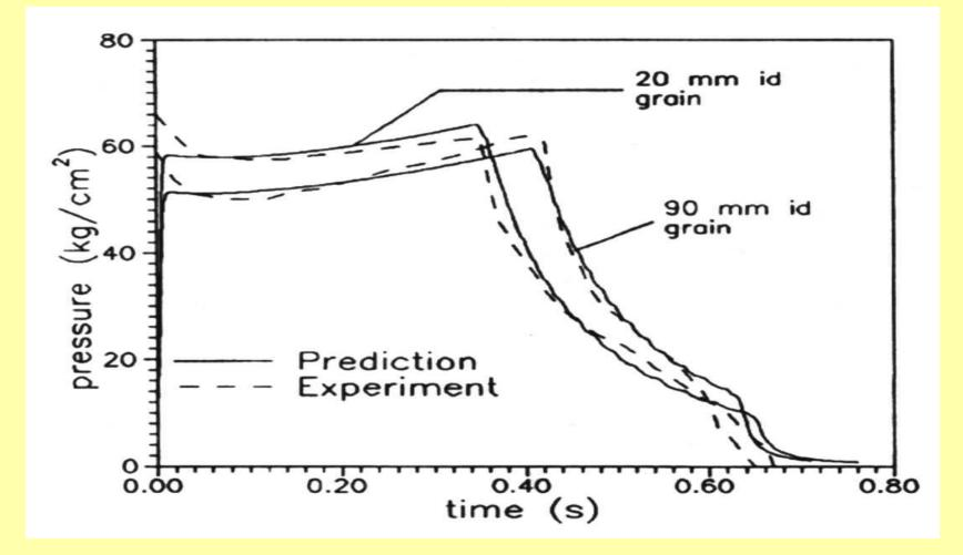
Proving the point: Predictions of pressure time curve of a highly loaded (implying significant erosive burning) solid motor and experimental data from a Japanese work.
