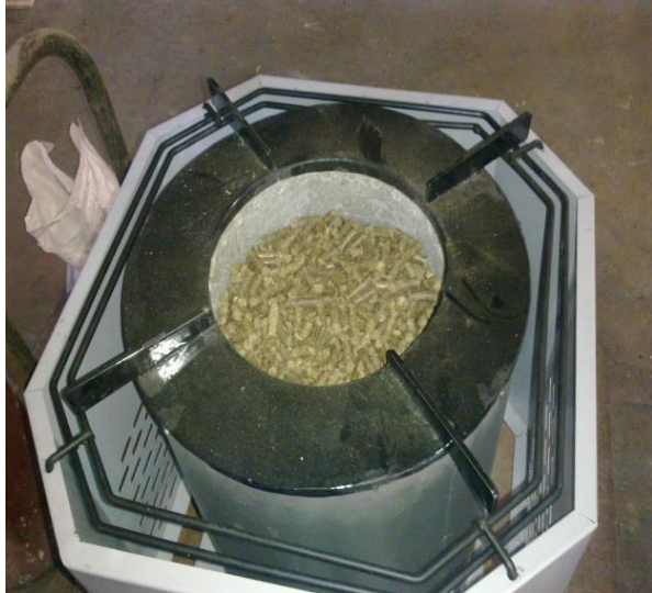
Gasifier based domestic pellet stove. Fan based Reverse downdraft Technology transferred to First Energy Pvt Ltd, Pune.
