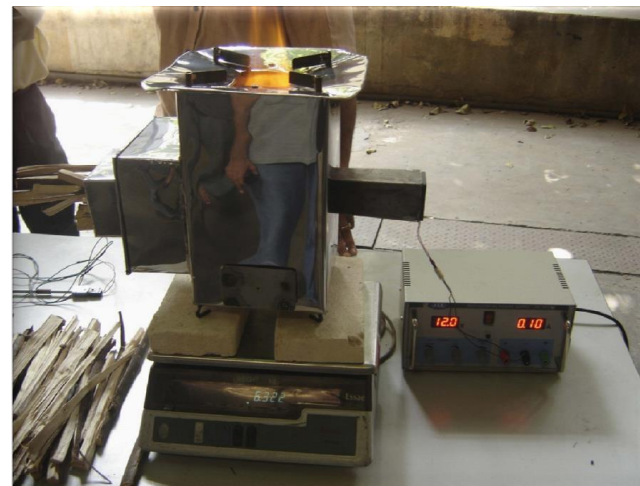
Horizontal domestic gasifier stove, Ejector induced gasification principle.
