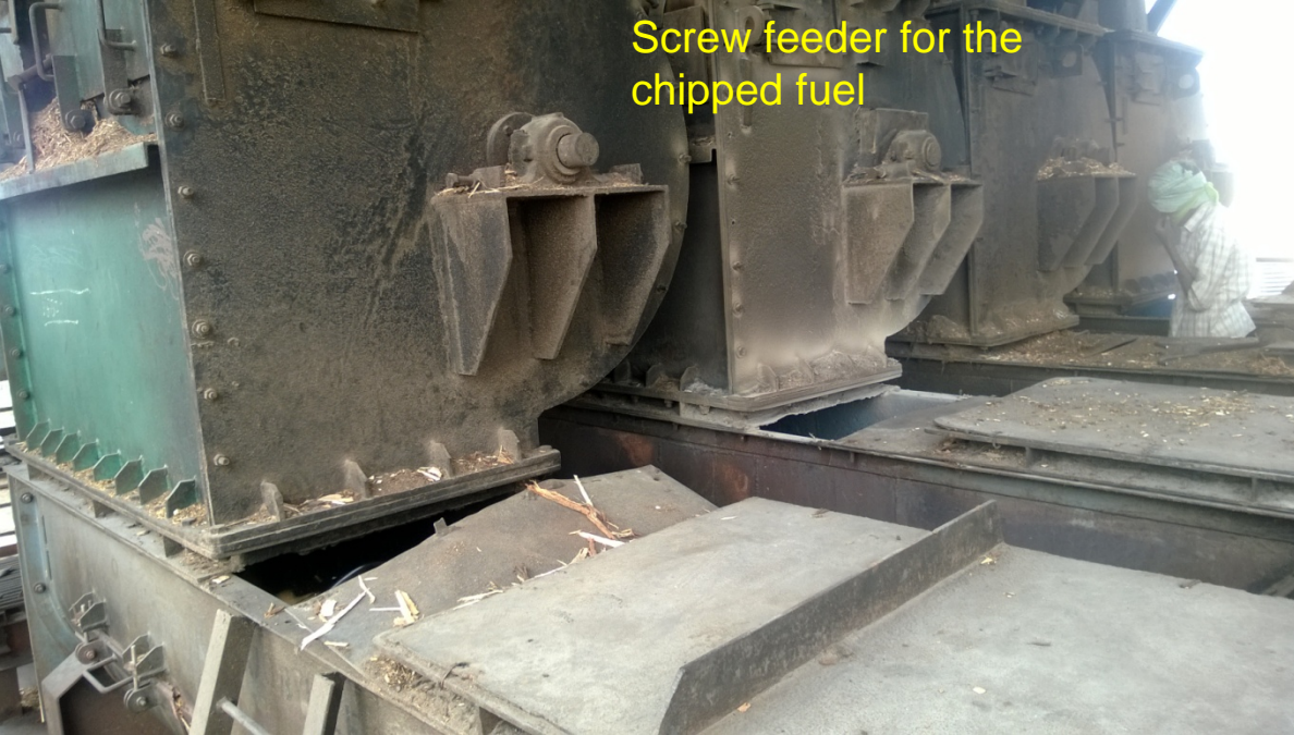
The chipped fuel is thrown to the outer region of the travelling grate that moves slowly towards the feeder
