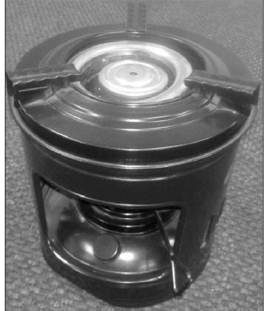
Premixed combustion of wick based kerosene stove, p = 1 \text{ atm} , T_0 = 300 \text{ K} M_0 \sim 0.0012
