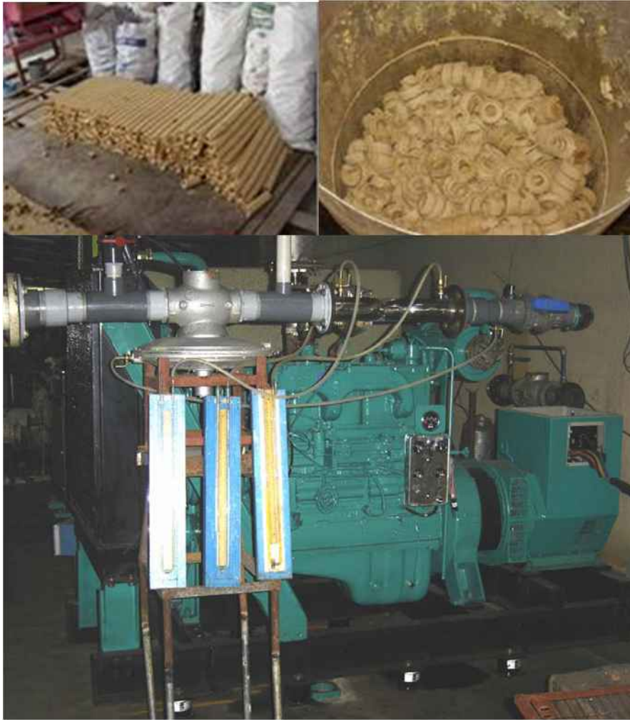
Figure 7.14: Experiments on gas engine working on the Japanese spiral rice husk briquettes
