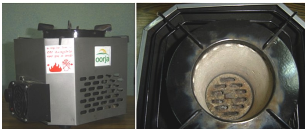
Figure 8.4: The pellet stove (a) notice the power pack towards the left bottom section of the left plate (b) the ceramic combustion chamber with grate at the bottom and secondary air holes towards the top
