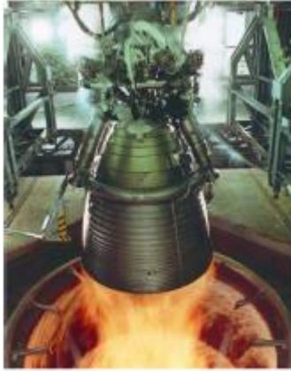
LOX - Kerosene based engine. Notice the bright exhaust
