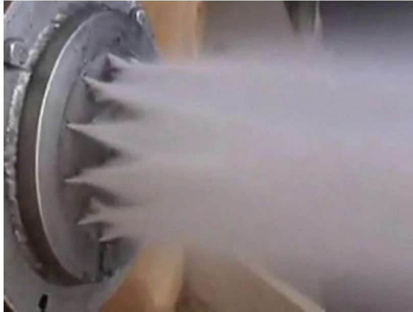
The spray from impinging injector head
