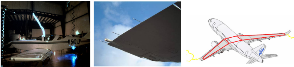
Figure 6.37.: The electrical discharge tests in a wind tunnel (left) and wing tip electrical discharge wicks on Boeing 737 aircraft (middle), electrical conduction paths on a wing with composite structure (right) (drawn from lightning, 2011 )
