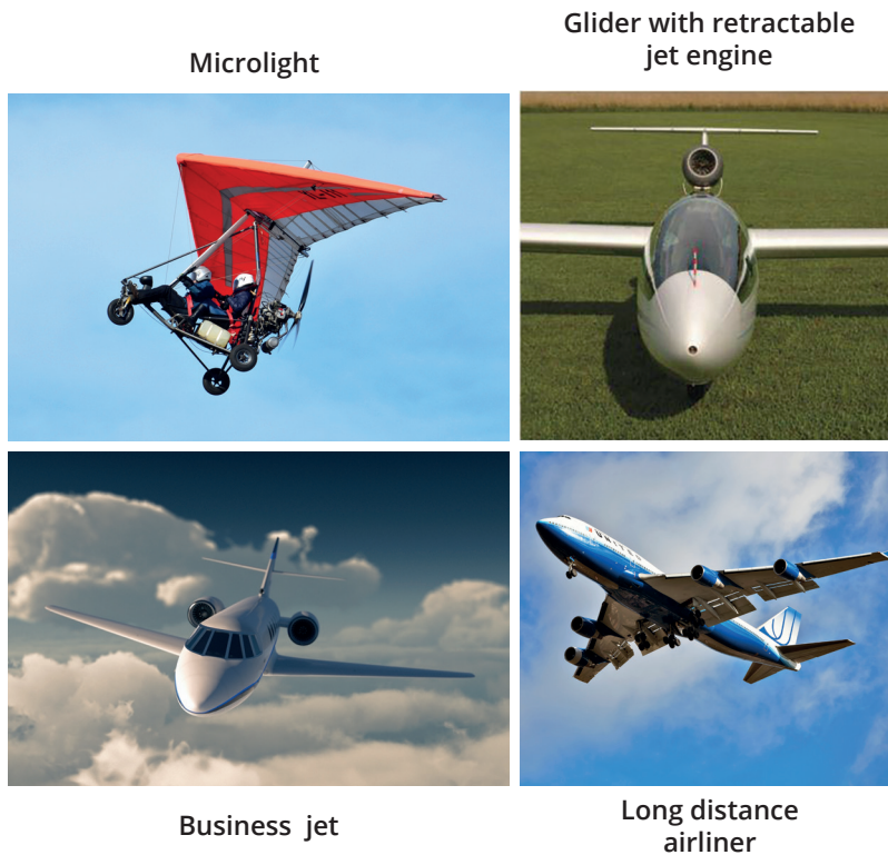
Figure 1.14.: Modifications of gliders to aircraft: The microlight that is a glider with an engine, a standard glider with a retractable engine, a business jet with slight sweep-back and a long range civil aircraft with sweep-back of about 45^\circ
