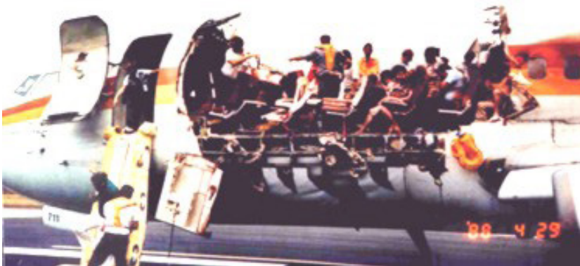
Figure 6.24.: The photograph of the crashed Boeing 737 air plane flown by Aloha airlines
