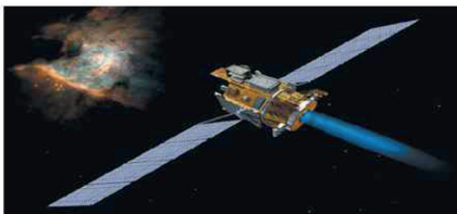
NASA's Deep Space 1 mission used an ion thruster for its primary propulsion. The engine operated at 2.3 kW producing a thrust of 0.09 N with I_{sp} of 3100 Ns/kg.
