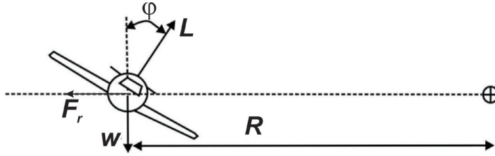
Figure 4.16.: Forces on an aircraft executing a coordinated turn
