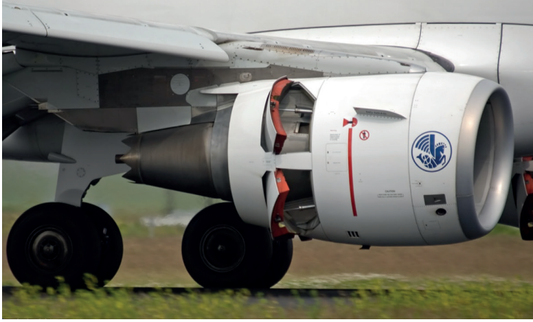
Figure 4.14.: The thrust reverser arrangement on a typical turbo-fan based engine. On the application of the reverser, the four flap doors open up covering a part of the exit area and directing most of the bypass flow laterally and in part in the forward direction; drawn from Wikipedia 5 , 2016
