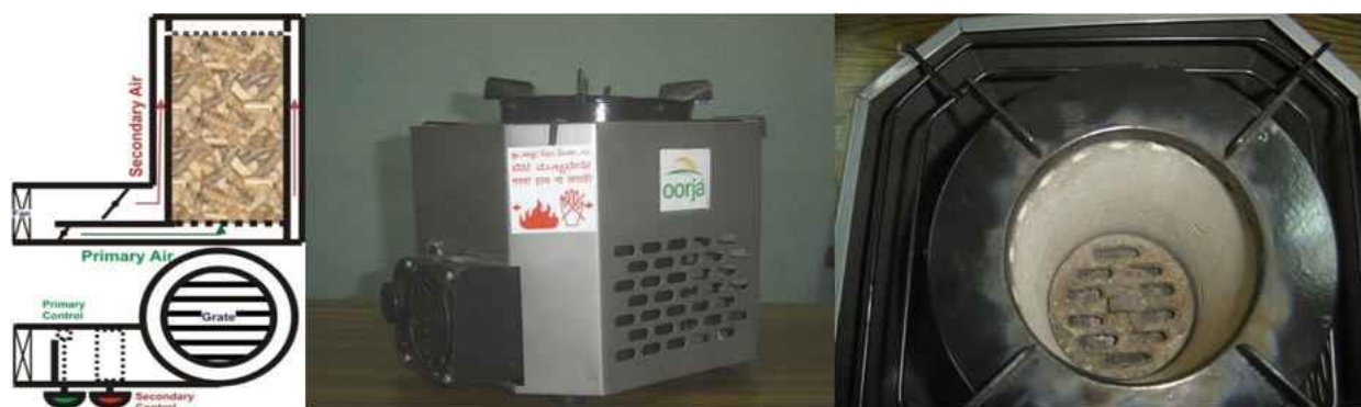
Figure 1: The reverse downdraft stove: fixed volume loaded pellet fuel (largely), gasification air supply from the bottom, combustion air from the top holes both needing a fan of 1.5 We for 3 kWth power.
