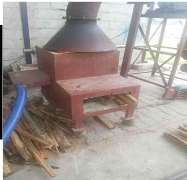
Figure 4. Stoves at 10 and 30 kg/h capacity in industrial use
