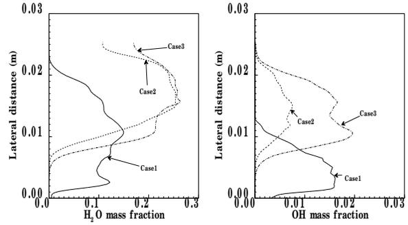
**Fig. 3 Comparison of mean profiles with various stream temperatures at  $x = 0.5$  m (a)  $H_2O$  mass fraction (b)  $OH$  mass fraction.**
