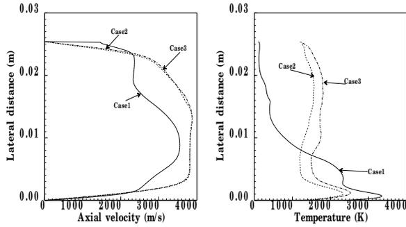
**Fig. 2 Comparison of mean profiles with various stream temperatures at  $x = 0.5$  m (a) Velocity (b) Temperature.**
