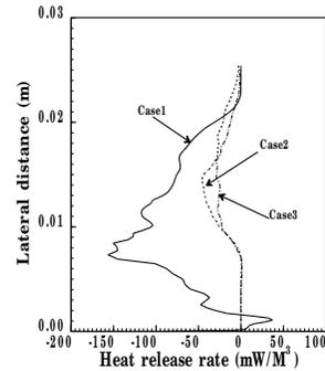
**Fig. 4 Comparison of heat release rate mean profiles with various stream temperatures at  $x = 0.5$  m.**
