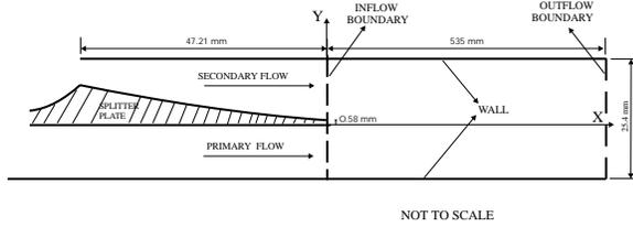
**Fig. 1 Schematic Representation of experimental setup of Erdos et. al.[11] for which computations were done**
