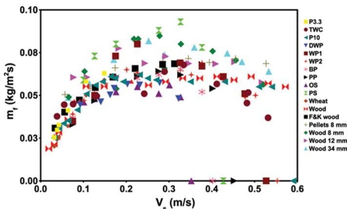
**Figure 1** Fuel consumption rate ( $m_f = \rho_p i$ ) with air superficial velocity. P3.3 – pellets (3.3% ash), P10 – pellets (10% ash), Wh – wheat, Wo – wood, from current work. WP1, WP2, BP, PP, OS, PS – Porteiro et al. (2010a). F&K – Fatehi and Kaviany (1994), P8 – pellets 8 mm, W8, W12, W34 – wood 8 mm, 12 mm, 34 mm – Ronnback et al. (2001). DWP – digester waste pellets – Gnanendra et al. (2012). TWC – Horttanainen et al. (2002). (Figure is provided in color online.)
