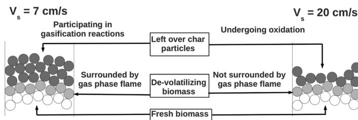
Figure 10 Schematic of the reaction zone at  $V_s = 7$  cm/s and 20 cm/s.
