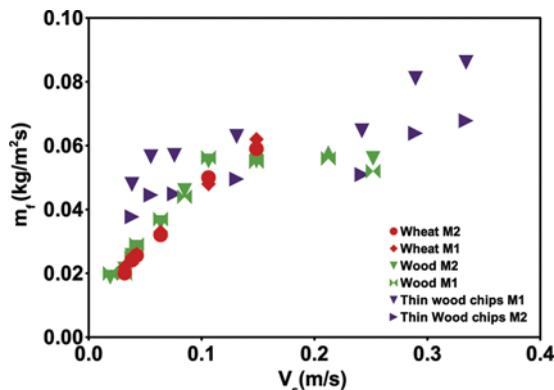
**Figure 3** Propagation rate estimated from two methods; M1 - method 1; M2 - method 2; note that thin wood chips show larger regression rate compared to dense biomass - wood and wheat. (Figure is provided in color online.)
