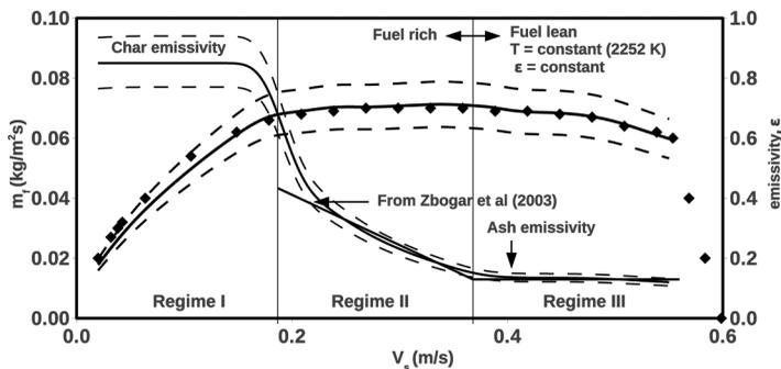
**Figure 12** Model results. Solid line: model results; dashed lines: fuel mass flux calculated by incorporating  $\pm 10\%$  uncertainty in emissivity; data points: experimental results; emissivity values with bounds and correlation of Zbogor and Frandsen (2003) are also shown.
