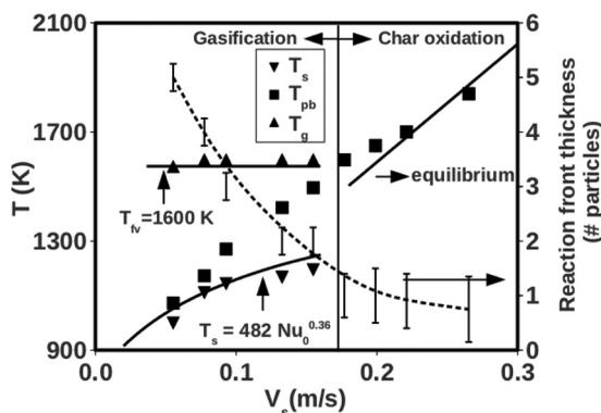
**Figure 9** Variation of gas, surface, and peak bed temperatures ( $T_g$ ,  $T_s$ ,  $T_{pb}$ ), reaction zone thickness with  $V_s$ . Solid lines -  $T_s = 482[K]Nu_0^{0.36}$  (model) in the gasification regime and equilibrium temperature in char oxidation regime and volatiles flame temperature ( $T_{f_1}$ ) = 1600 K in gasification regime. Data points are from experimental results. Dotted line represents the mean behavior of reaction zone thickness,  $\delta_f$ .
