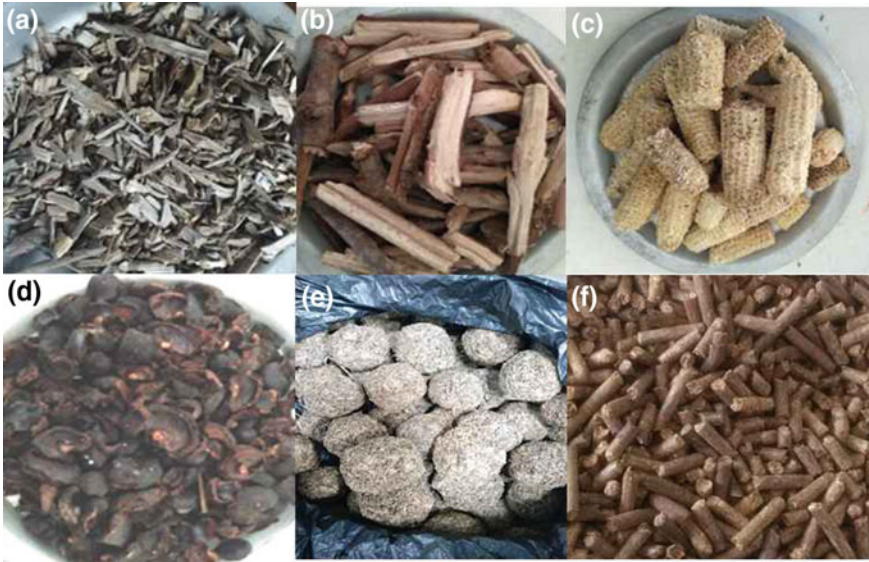
Fig. 3 Fuels that can be used in HC3D combustion systems: a cut tree droppings along with bark, packing density of 200 to 210 kg/m 3 , b cashew chopped pieces, packing density of 240 to 280 kg/m 3 , c corncobs, packing density of 200 to 210 kg/m 3 , d cashew shell waste—90 to 100 kg/m 3 , e processed sawdust–cowdung balls, 60 to 80 kg/m 3 , f pellets of a mix of seasonal agro-residues, packing density = 600 kg/m 3 , ash content of all biomass ≤ 5%
