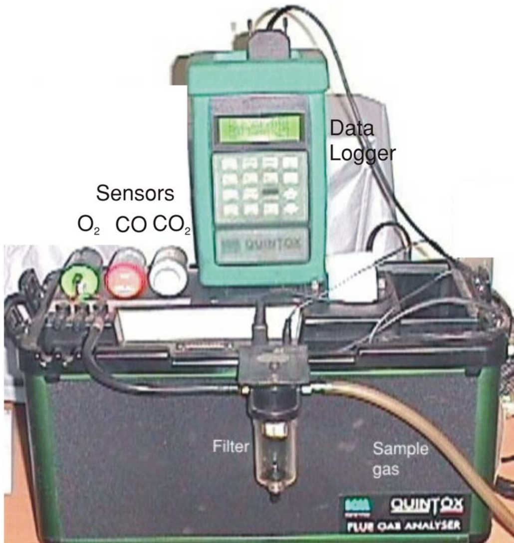
Figure 2.6: Quintox analyzer used for composition measurement.
