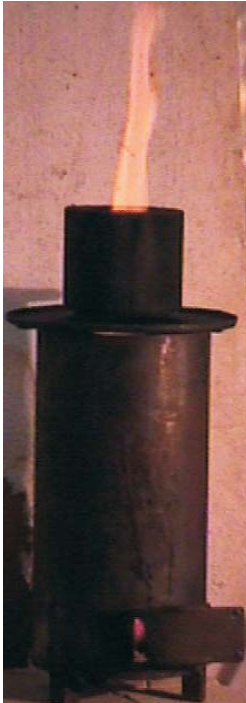
Figure 3.29: A photograph of 40 mm diameter AR = 6 stove functioning at 2.3 kW power level.
