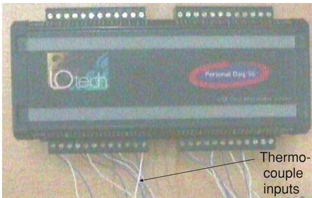
Figure 2.9: Personal daq USB based data acquisition system.
