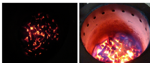
Figure 4.1: Photographs of wood char combustion (left) and pellet char combustion (right) in the stove
