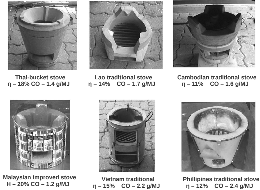
Figure 1.2: Several designs of mud, clay and ceramic stoves from Indo-Chinese countries tested by Bhattacharya et al. (2002)
