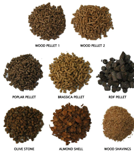
Figure 2.2: Photograph of all the biomass used by Porteiro et al. (2010a)
