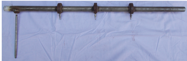
Figure 2.12: 5 mm tube attached perpendicular to the 42 mm tube.
