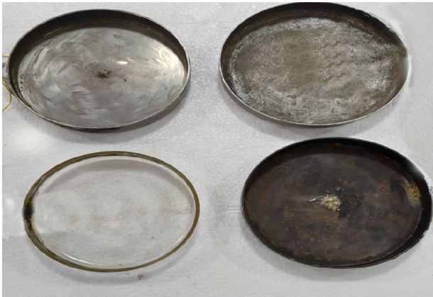
Figure 1. Pans of 200 mm dia, 40 mm depth made of stainless steel (SS), mild steel (MS), aluminum alloy (AL) and glass (GL) (clockwise from the top) on left side and pans of 300, 400 and 500 mm dia, 40, 50 and 60 mm depth made of MS on the right side.
