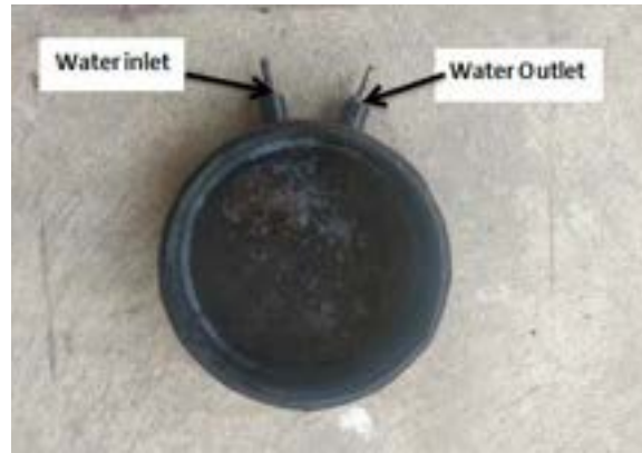
Figure 3.4: Jacketed pan circulating water at ambient temperature in the jacket
