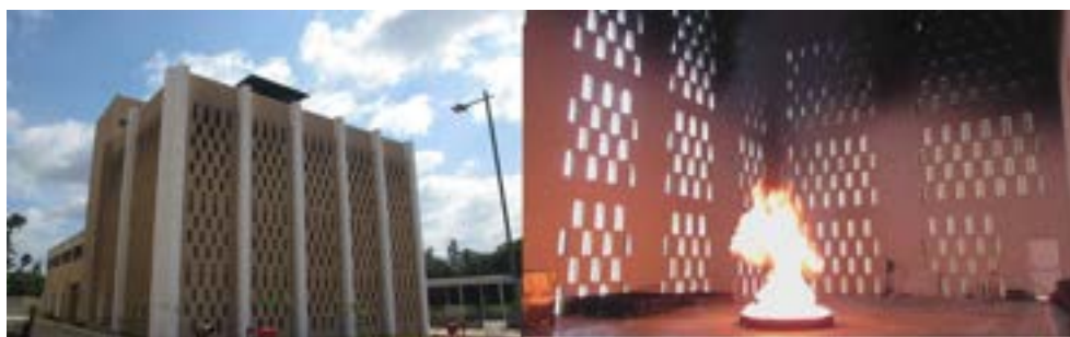
Figure 2.6: Indoor fire laboratory - On the left is the outside view. On the right is the 2\text{ m} circular pan fire burning inside the laboratory.
