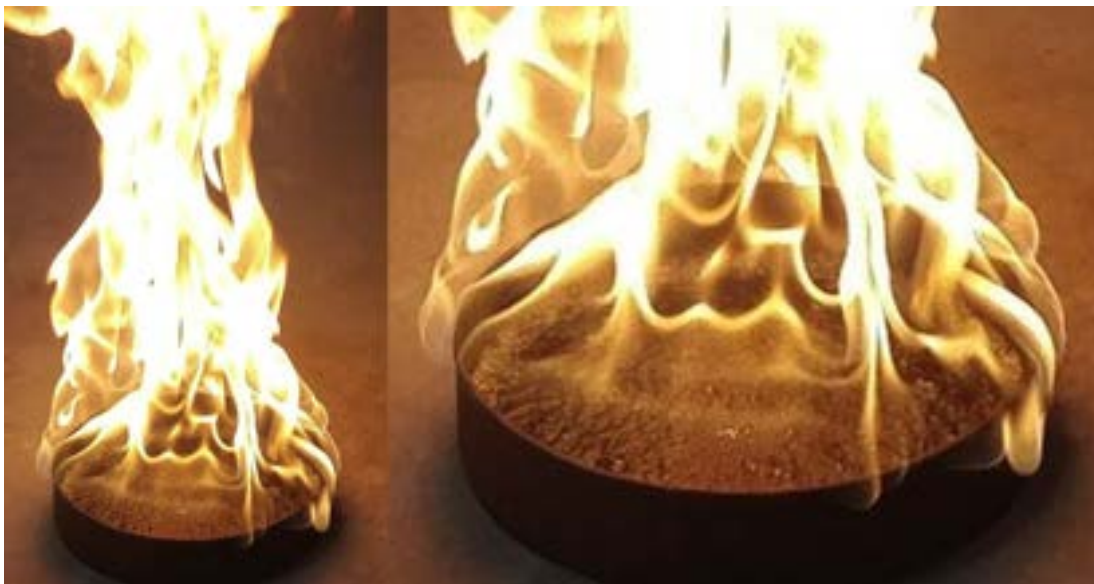
Figure 3.10: The 0.2 m MS pan with n-heptane undergoing vigorous pool boiling. The right side photograph is an expanded version of the left side photograph
