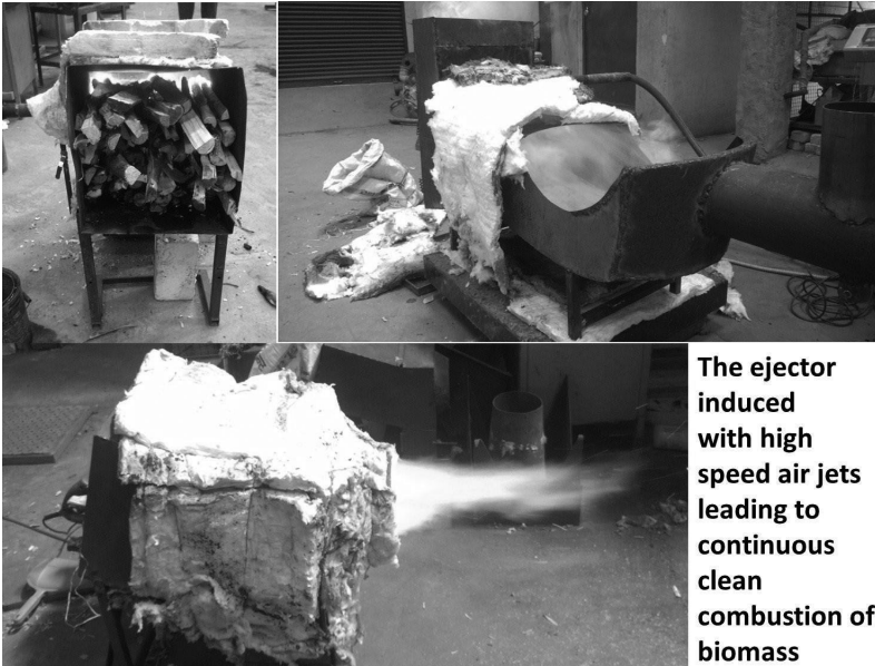
Photo 19.14 The development of an ejector based horizontal clean combustion system, 2015
